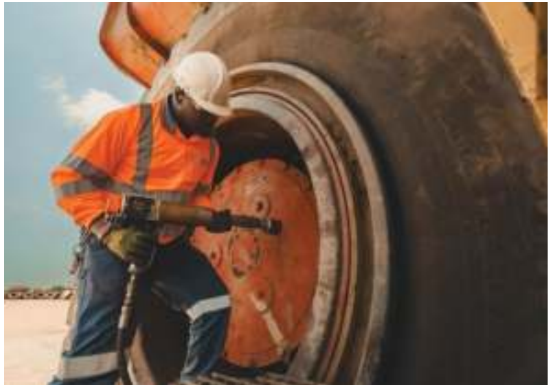
Servicing mining tyres—particularly earthmover tyres weighing nearly 5 000 kilograms—has always posed a significant risk.
